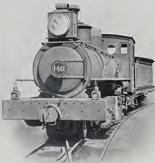
THIS PICTURE SHOWS ONE OF THE LATEST ANTOFAGASTA LOCOMOTIVES, AND THE DIFFERENCE BETWEEN THE 2' 6" GAUGE AND THE ORDINARY ENGLISH STANDARD GAUGE OF 4' 8 1 / 2 "
